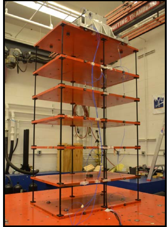
Figure 1: 6 Story Base Structure with NES attached
